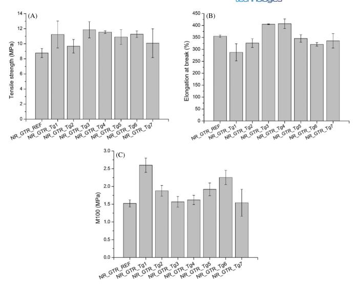
FIGURE 5 The (A) tensile strength, (B) elongation at break, and (C) M100 of the vulcanizates produced with the Taguchi method.
