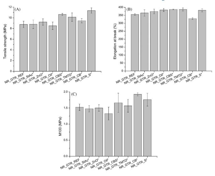
FIGURE 2 The (A) tensile strength, (B) elongation at break, and (C) M100 of the vulcanizates used in the first optimization process.
